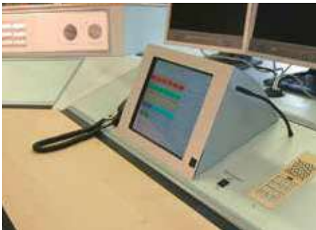
Tilt adjustment for built-in monitors
